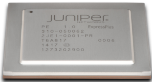
Figure 1: The custom-built Juniper Q5 ASIC
