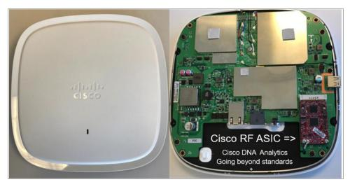
Catalyst 9120i with the Cisco RF ASIC chip
