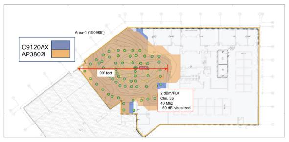
Comparison of C9120 and AP3802i coverage patterns as measured over the air
