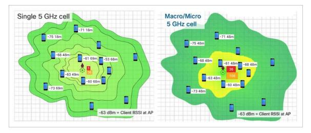
In the figure above, (on the left) a single channel cell, say channel 36, has a channel utilization of 60% because all clients are connected to that one channel. To make matters worse, they connect at nonuniform speeds, as the close-in clients connect much faster than the far-away clients.
