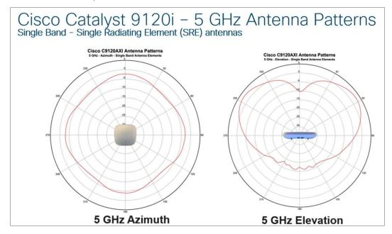
9120i secondary 5-GHz single-band antenna patterns
