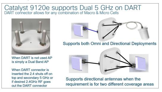
9120e antenna system using the DART connector for dual 5 GHz
